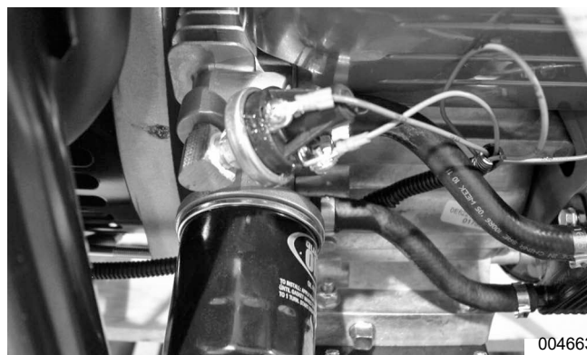
Figure 4-23. Low Oil Pressure Switch
